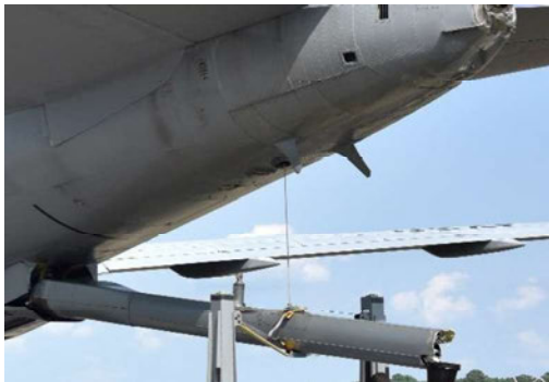
Remaining portion of boom (Tab S-5).
