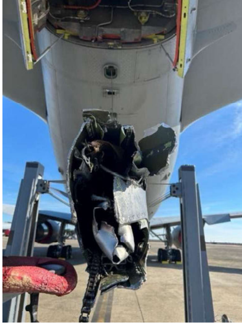
Break point of boom (Tab Z-3).
