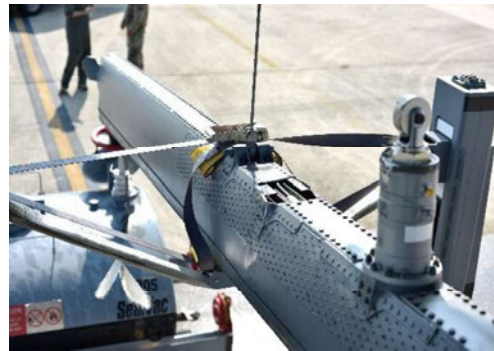
Missing latch hook eye (Tab S-14).
